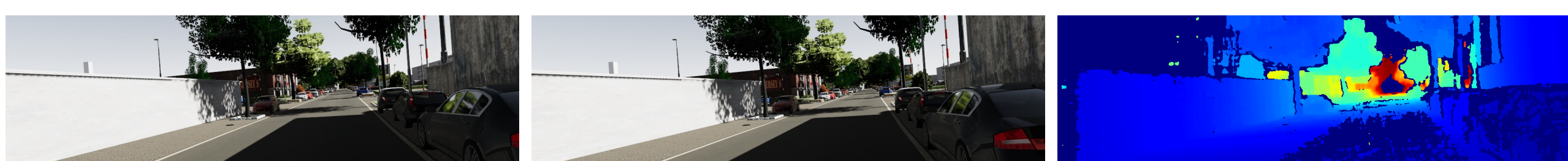
Fig. 3: Depth maps generated by SimSense using the stereo images exhibit the noise and incompleteness typical of real-world depth maps which helps to reduce the sim-to-real gap.
